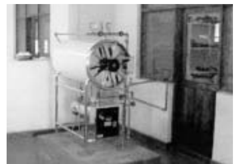
The new autoclave (for sterilizing equipment) at Mulanje Hospital, provided through MBF, is "crucial to the successful running of the hospital," according to Dr. Sue Makin.
